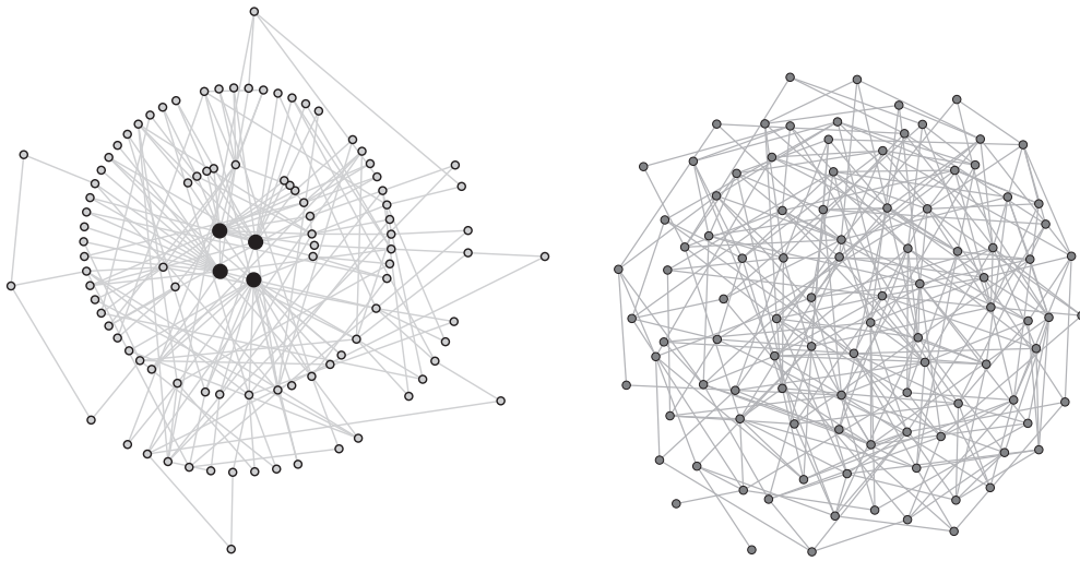
Figure 1. Illustrations of a BA network (left) and an ER network (right), both with n = 100 . BA networks have a high heterogeneity in the node's degrees as represented by the four bold nodes. While the mean degree of such a BA network is around 4, each of the bold nodes has over 25 connections.
