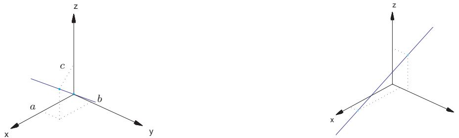
Figura 4.12: Retas (x, y, z) = (at, bt, ct) e (x, y, z) = (x_0 + at, y_0 + bt, z_0 + ct)
