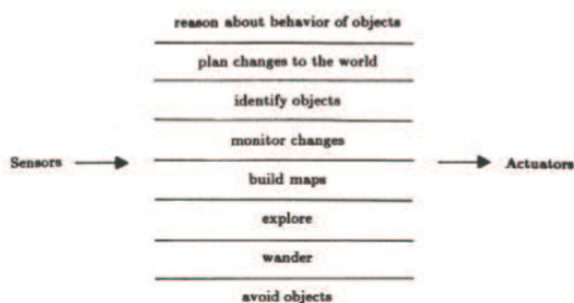
Figure 1. A traditional decomposition of a mobile robot control system into functional
