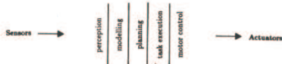
Figure 1. A traditional decomposition of a mobile robot control system into functional
