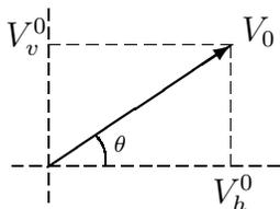
$$\begin{aligned} V_v^0 &= V_0 \sin \theta, \\ V_h^0 &= V_0 \cos \theta. \end{aligned}$$
